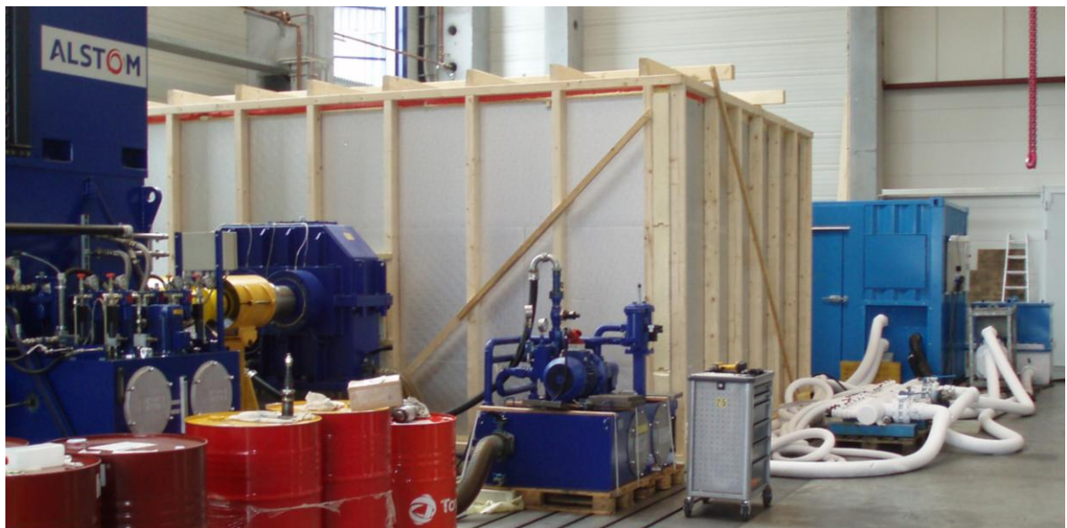
Picture 1: Test field with isolated WinDrive and cooling unit
