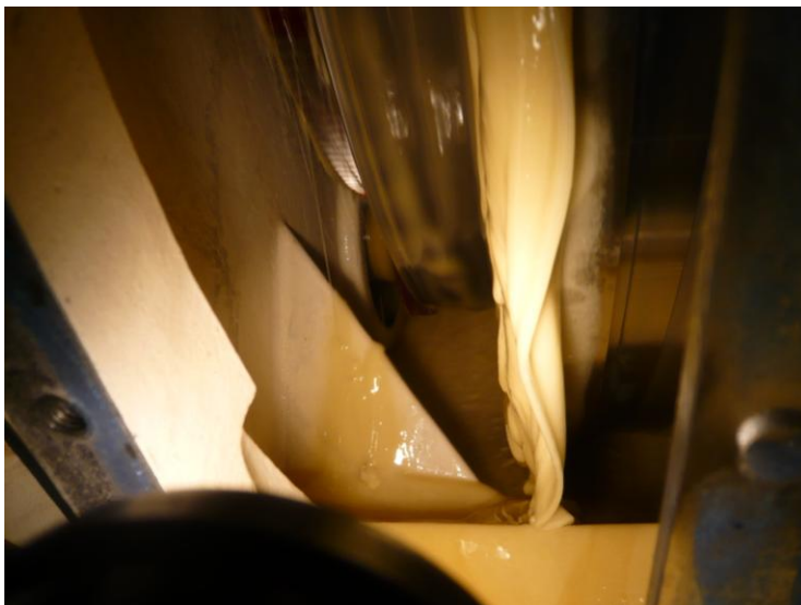
Picture 3: Gearbox oil at -30 °C (-22°F)
