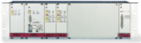
Fig. 3: Voith micro-processor control as 19" plug-in unit in control panel.
